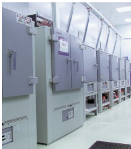
Chamber Ovens – Over 3000 cubic feet of oven capacity is dedicated to long term thermal bias age testing. The ovens take material to temperatures above Tg. At selected intervals, samples are removed and tested to verify material integrity.
