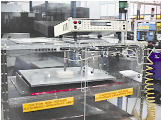
"Proof Test" fixture to test etched panels during fabrication process
