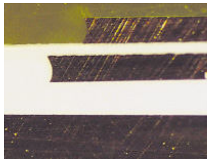
Cross sectional view of heavy copper - two-layer 10 oz. over 10 oz. utilizes Thermal Clad HT dielectric with a 0.020" (0.5mm) copper base.
